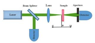
Fig. 1: Schematic diagram of the experimental setup for closed aperture z-scan technique.
