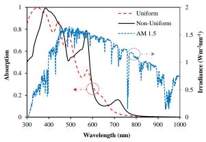
Fig. 4: Overlap figure of the absorption intensity and the radiation intensity of the sun spectrum (AM1.5).
