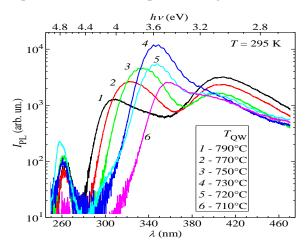
Figure 2: RT PL spectra of InAlN/AlGaN MQWs grown at different TQW.
