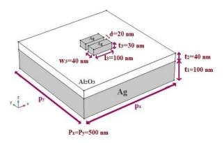
Fig. 1: The unit cell of the proposed PPA biosensor structure.
