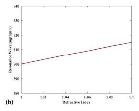
Fig. 2: (a)The structure absorption spectrum,(b) The resonance peak wavelength curve; for various refractive indices of the analyte.
