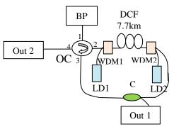
Figure 1: The proposed experimental setup for the MBRFL generation.
