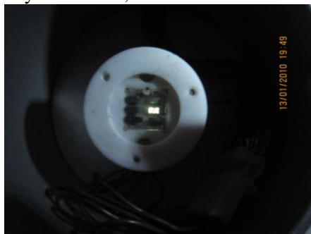
Figure 2. Illumination from the white OLED, based on the combination of prime blue emission and the complementary orange emission.
