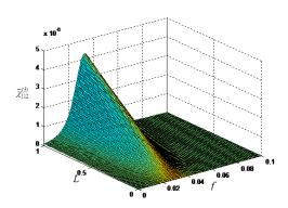
**Fig. 1.** Variations of the effective third-order nonlinear susceptibility coefficient  $(\bar{\chi}_{112}^{(3)})$  after addition of gold ellipsoidal nanoparticles for a degenerate four-wave mixing at 532 nm wavelength on the basis of L and f
