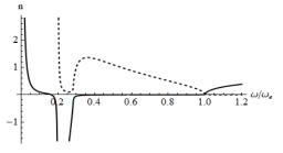
Figure 3. The plot of refractive index of the metamaterial as a function of frequency, the real parts (solid lines) and imaginary parts (dashed lines).
