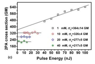
Figure 1. 2PA cross section versus pulse energy for B3FL (a), M2CMK (b) and 3C (c)
