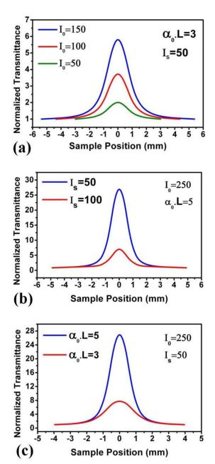
Figure 1. Simulation of Z-scan curves for a saturable absorber material. (a) For different on-axis peak intensity  $I_0$ , (b) for different saturation intensity  $I_s$  and (c) for different values of  $\alpha_0 L$ . ( $I_0$  and  $I_s$  have the same arbitrary unit)
