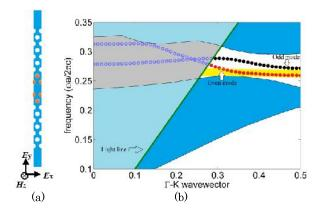
Figure 1: a) Top view of the super cell, b) TE polarized ( $H_2 E_{\nu}$ ) band structure for W09 waveguide in  $\Gamma$ -K direction (r=0.3a).
