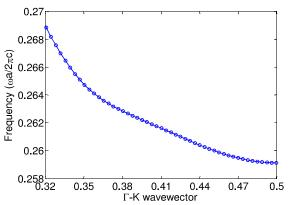
Figure 2: Fundamental even band of the W09 waveguide filled with Si<sub>3</sub>N<sub>4</sub>.
