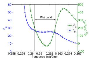
Figure 3: Calculated group index  $(n_g)$  and group velocity dispersion  $(\beta_2)$  values of even fundamental mode depicted in Fig. 2.
