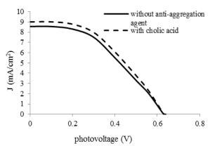
Figure 2: Current density-voltage characteristics for dye in the absence and presence of anti-aggregation agents
