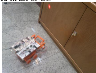
Figure3. The hardware system contains of a four wheel chassis with a rolling arm on the head
