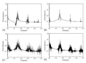
Fig. 6. Power spectrum for oscillations of excited dark hexagons in 2C = 31.30 (a), 2C = 31.50 (b), 2C = 31.70 (c) and 2C = 31.90 (d).
