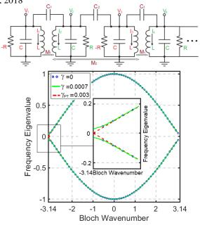
Figure 2: (a) The circuit model of the structure consists of a coupled LRC oscillator, one with -R for gain material and the other with R for loss material. Mutual inductances  $(M_1,M_2)$  and capacitive  $(C_1,C_2)$  coupling are included for generality. (b) Normalized dispersion diagram for various  $\gamma$  values. At  $\gamma = \gamma_{PT}$  the gap between the two bands disappears. The inset shows a zoomed-in portion of the figure about the zone edge.
