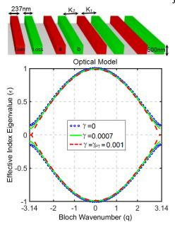
Figure 1: (a) PT array structure with intra- and interdimer coupling  $K_1$  and  $K_2$ . Sublattices cuboid of aand b are gain and loss materials. Dimensions are designed in such a way that all of the waveguides are single mode. (b) Normalized Dispersion diagram for various  $\gamma$  values.
