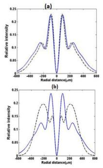
Figure 1: Intensity distributions of BG ( $J_1$ ) beams versus radial distance for  $\underline{z=10}$  cm from the laser aperture for p=5W,  $\alpha$ = 720 m<sup>-1</sup>, K=10.5 $\frac{W}{K.m}$  and  $\delta_p$  = 200  $\mu$ m for a) p=1W b) p=5W. Solid plots represent the nonthermal BG beam, dashed plots shows thermally-affected BG beam.
