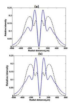
Figure 4: Intensity distributions of BG beams versus radial distance for  $\underline{z=10~\text{cm}}$  for p=5W,  $K=10.5\frac{W}{K.m}$  and  $\delta_p=200\,\mu m$  **a)**  $\alpha=520~\text{m}^{-1}$  **b)**  $\alpha=920~\text{m}^{-1}$ .
