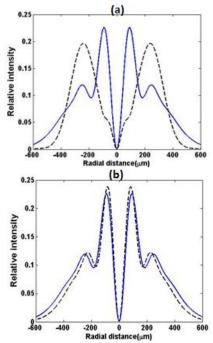
Figure 2: Intensity distributions of first-order BG( $J_1$ ) beams versus radial distance for  $\underline{z=10~cm}$  for p=5W,  $K=10.5\frac{W}{K.m}$  and **a)**  $\delta_p=100\,\mu m$  **b)**  $\delta_p=300\,\mu m$ .
