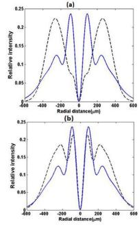
Figure 3: Intensity distributions of BG ( $J_1$ ) beams versus radial distance for  $\underline{z=10~cm}$  for p=5W,  $\alpha=720~m^{-1}$  and  $\delta_p=200~\mu m$  for **a**) K=9 $\frac{W}{K.m}$  **b**) K=12 $\frac{W}{K.m}$ .
