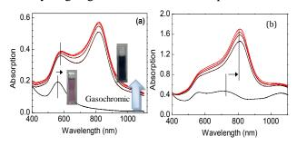
**Fig.4:** (a) Spectral time variations of Au-Mo oxide samples in the gasochromic process for Mo:Au ratios of 10:1 and (b)sample of 40:1, at hydrogen (10%) injection time intervals of 15 min.
