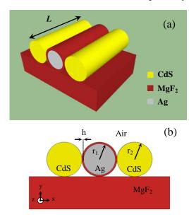
Figure 1: (a) Three dimensional schematic of the spaser (b) Cross-sectional view of the SIMIS structure.
