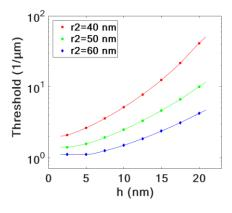
Figure 4: Lasing Threshold of SIMIS based spaser as a function of h for  $L = 30 \mu m$  and three different values of r2.
