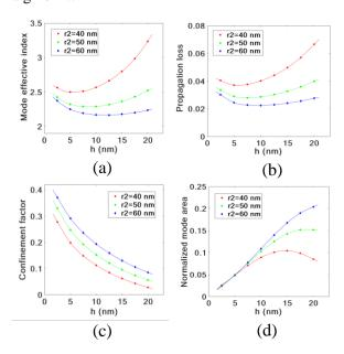
Figure 3: (a) Mode effective index (b) Propagation loss (c) Confinement factor (d) Normalized mode area of hybrid plasmonic mode in SIMIS structure.
