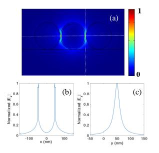
Figure 2: Normalized electric field (a) cross section distribution (b) x component (c) y component of propagated hybrid plasmonic mode in SIMIS structure.
