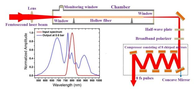
Figure 1. Schematic setup used for WLC generation in order to produce sub-8 fs pulses
