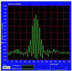
Figure 4. Interferometry Autocorrelation measurement showing 8 fs pulses.
