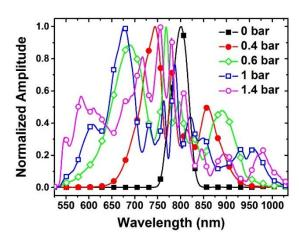
Figure 2. WLC spectrum at different gas pressure
