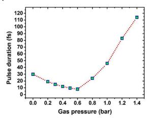
Figure 3. Pulse duration of compressed pulses
