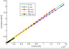
Figure 3. The luminous-current curves for different perovskite thicknesses.
