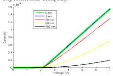
Figure 2. The I-V curves for different perovskite thicknesses.
