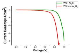
Figure 3. Dark current-voltage characteristic of solar cells with/without  $Al_2O_3$
