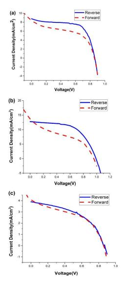
**Figure 2** Current-voltage characteristics of solar cell (a) without  $Al_2O_3$  (b) with  $Al_2O_3$  (c) with  $Al_2O_3$ / without spiro-OMeTAD
