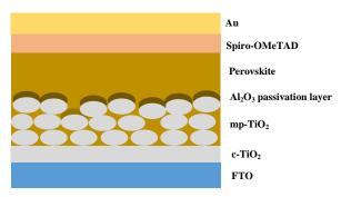
**Figure 1** Schematic of perovskites solar cell with  $Al_2O_3$ .
