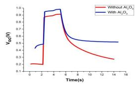
Figure 4. Photovoltage decay characteristics of devices with/without  $Al_2O_3$
