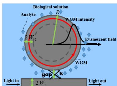
Fig. 1. A photonic WGM disk resonator based biosensor
