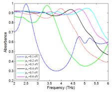
Fig. 4: Absorbance spectra at various chemical potential.
