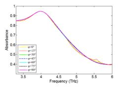
Fig. 3: Absorbance spectra at different azimuthal angle φ.
