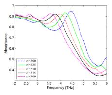
Fig. 5: The effect of substrate dielectric constant on the absorbance spectra of THz metasurface.
