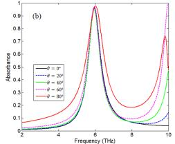
Fig. 3: The absorbance spectra of the MA at different angles of incidence for (a) TE and (b) TM waves.
