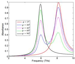
Fig. 4: The absorbance spectra of the MA for different polarization angles.
