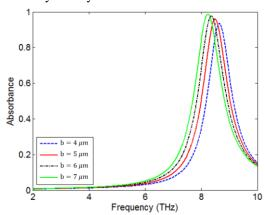
Fig. 5: The absorbance spectra of the MA for different long axis radii of the elliptical patches.
