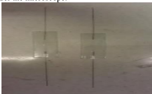
Figure 3: Experimental tapered optical fiber liquid cell
