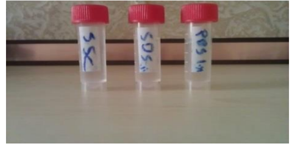
Figure 5: Three biological buffers used for measurement of refractive index change: SSC, SDS, PBS
