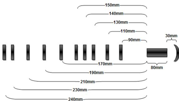
Figure 3 : Investigated plano-concave resonators with different length
