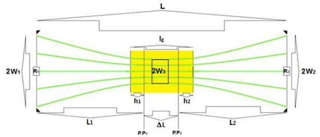
Figure 1: Schematic of a typical active resonator
