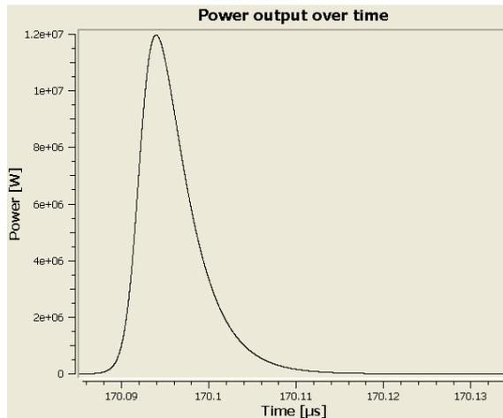
Figure 6 : time profile of laser output pulse
