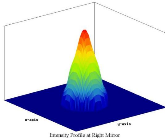
Figure 5: TEM<sub>00</sub> Q-Switched output pulse from optimized simulated resonator
