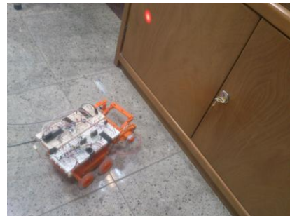
Figure3. The hardware system contains of a four wheel chassis with a rolling arm on the head
