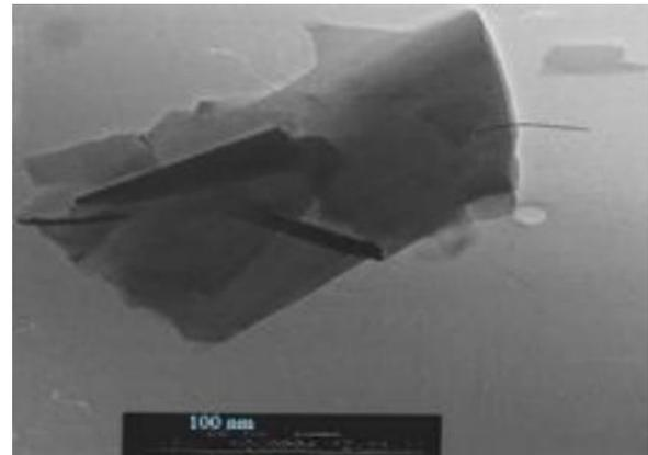
Figure 1: TEM image of graphene synthesized in nitrogen
