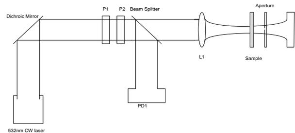
Figure 2 : experimental setup of closed aperture Z-scan
