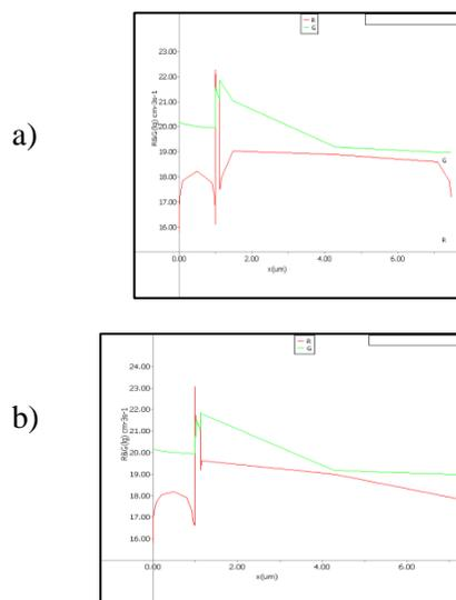
Fig. 5. R&G characteristics of CdS/CdTe solar cells a) without buffer layer, b) with Buffer layer
