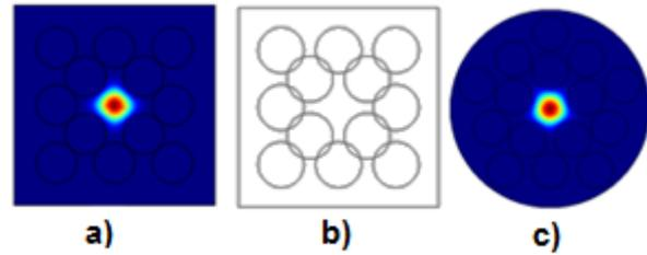
Fig.3 The 2D (two dimensional) intensity distribution of PCFs with square and penta – lattice while a)  $d/\Lambda = 0.7$ , b) and c)  $d/\Lambda = 0.8$ , respectively
