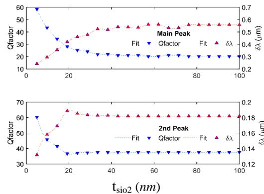
Fig. 4: Left hand side of the figure illustrates  $Q$ -factor of the BPF studied versus different  $t_{SiO_2}$  sizes while the right hand side investigates the FWHM ( $\delta\lambda$ ) for: (a) larger peak of (b) weak peak.  $\mu_c = 0.36$  eV. Dashed lines represents the spline fit function applied to discrete points.
