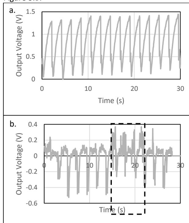
Figure 3. Output voltage of rGo/Ag NPs decorated TENG.
