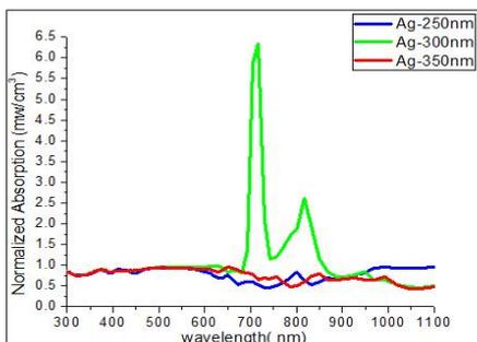
Figure2: absorption for three periods of 250nm, 300nm and 350nm for silver Nano rod in active region.
