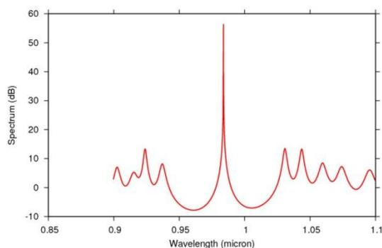
Figure 2: 980 nm VCSEL mode spectrum
