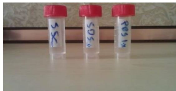
Figure 5: Three biological buffers used for measurement of refractive index change: SSC, SDS, PBS
